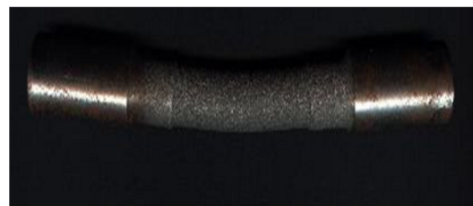
(b) Bent coated specimen with a thin layer
